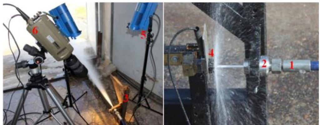
**Figure 9.** Measuring stations for recording images of impulse and continuous water jets operating in the air medium: 1—high-pressure power cord, 2—self-excited pulse head, 3—head mounting bracket, 4—force sensor, 5—lighting, 6—Phantom V12.1 camera.
