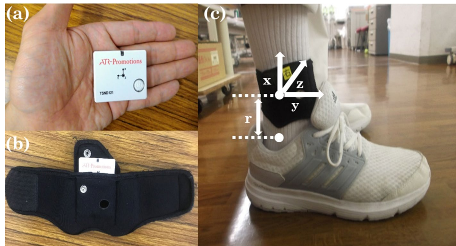
Figure 1. Configuration of the IMUs. (a) The IMU with the accelerometer and gyroscope. (b) The special band for wearing the IMU on the shank. (c) The position and coordination of the IMU. Two IMUs are attached to the shank just above the malleolus at a distance of r . IMUs are attached to the shank in the position 0.03 m above the malleolus. The axes x , y , and z are the coordinate system of the IMU, where the z -axis is perpendicular to the sagittal plane formed by the y and z -axes.
