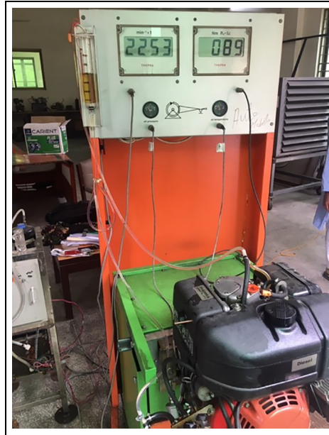
Figure 3. Engine mounted on Thepra test bed.
