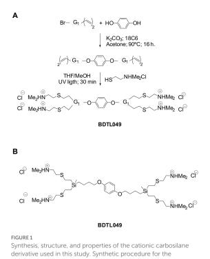
formation of compound BDTL49 (A) and its corresponding chemical structure (B). G1 denotes first generation of the carbosilane scaffold. Molecular weight of 964 Daltons. The compound is air and water stable, soluble in protic solvents like water or methanol, and non-soluble in organic solvents. TABLE 1 Minimal inhibitory concentration (MIC) and minimal bactericidal concentrations (MBC) of depicted antibiotics against B. subtilis W168.
