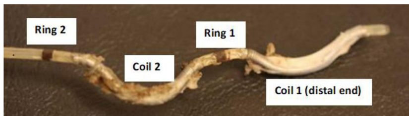
FIGURE 2 Extravascular implantable cardioverter-defibrillator (EV ICD) tissue capsule. Extracted EV ICD lead (2 years) showing representative tissue capsule [Color figure can be viewed at wileyonlinelibrary.com ]
