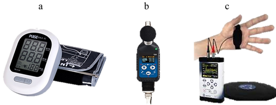
Figure 1. a) Pulse GALA X for measuring BP and HR; b) Svantek 104 for measuring noise exposure; c) Svantek 106A for measuring WBV and HAV.
