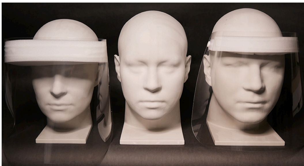
Fig. 3. 3D printed ISO headforms mounted with face shields. The small (left, with an ENT face shield), medium (middle) and large (right, with a standard face shield) headforms are representative of the head size groups of the population, and were used to gauge the length of face shield strap required to accommodate the range in head sizes.
