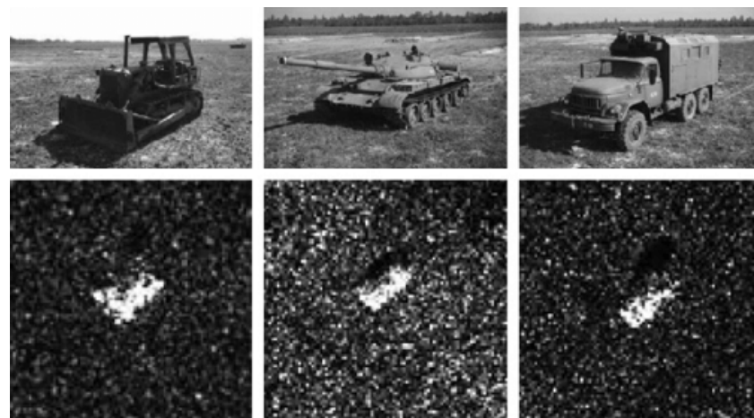
Figure 6. Camera images and corresponding SAR images from MSTAR database [42].
