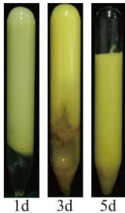
Figure 1. State of the gel prepared from 0.6 wt% HPAM and 0.6 wt% WAPR after aging at 110 °C for 1, 3, and 5 days.
