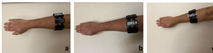
Figure 3. Three armband sensor positions to test the effect of sensor position on data quality: (a) rotated, (b) standard, and (c) slid down.
