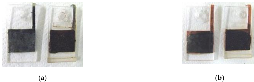
Figure A2. Images of vulcanized MCF rubber on anode by electrolytic polymerization: (a) stainless electrodes; (b) copper electrodes; right is the cathode and the left is the anode.
