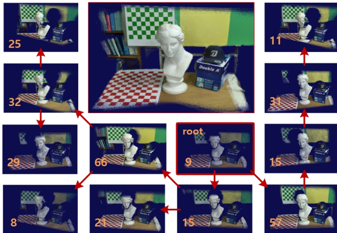
Figure 6. Merge of separate components. When the similarity graph method was applied to an input stream of 843 frames with \tau_{good} = 0.75 , we obtained 12 separate components. To combine them as much as possible, we first repaired each component using \tau_{repair} = 0.8 , and built a component graph whose edges are those with the highest similarity measure between the components. Then, after finding a maximum spanning tree each of whose vertices are shown in the small figure with its frame number, we performed the component-wise camera tracking with \tau_{fair} = 0.6 while traversing the tree, computing the rigid transformations between the components. As a result, we could collect all components into a common space as shown in the large figure. Note that only 319 frames out of 843 were actually used to reproduce the final geometry.
