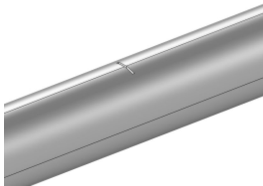
Figure 21. Cable sheath with 10% section loss rate.
