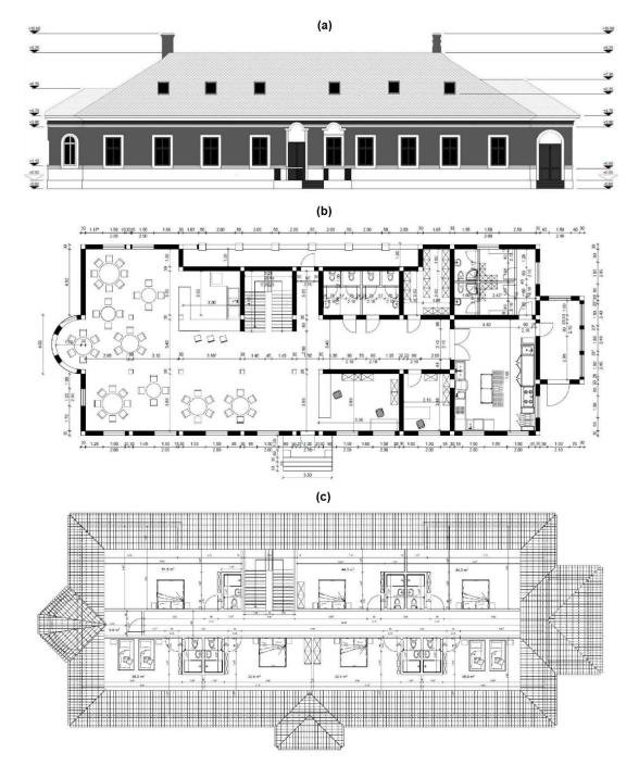
**Figure 12.** Proposed rehabilitation and restoration; (**a**) Reconstructed facade; (**b**) Envisioned ground floor; (**c**) Envisioned attic.
