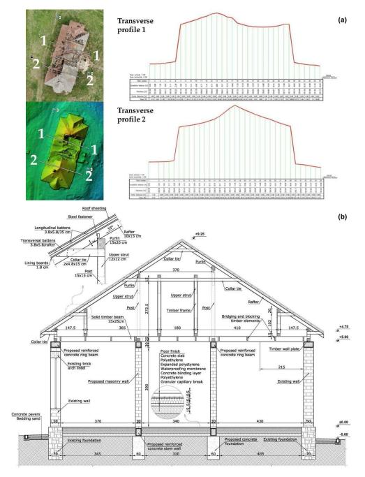
Figure 13. (a) Extracting metric data from transverse profiles; (b) Envisioned section.
