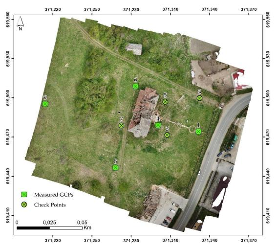
Figure 10. Obtained orthophoto.
