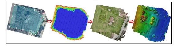
Figure 6. Photogrammetry processing stages.
