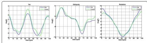
**Figure 2 Technical comparison by triangular plate.** Superimposition of the estimated angles provided by the F4A (blue lines) and the corresponding reference angles calculated with the markers on the associated triangular plate (green lines), as recorded during one typical trial of a randomly selected subject, for each of the three anatomical axes (three plots). This technical comparison was made in the reference frame of the three marker cluster.
