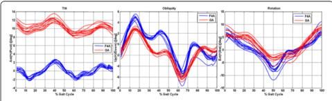
**Figure 3 F4A versus GA: intra-subject repeatability.** Pelvic angles about the three axes provided by F4A sensor (blue lines) as the mean of all the gait cycles detected, and by the GA system (red lines), expressed in the laboratory reference frame; for both, 10 repetitions of the right leg are superimposed, for the same representative subject. Just for this comparison, static angles were not added to F4A data.
