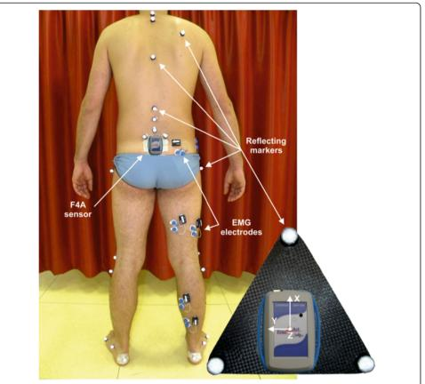
**Figure 1** The marker set and F4A sensor positions on the sacrum in a representative subject. Image taken from the experimental session. Electrodes for EMG signal data collection can also be seen, though not addressed in the present study. The inset shows the triangular rigid plate with the three marker cluster and the F4A with its reference frame bonded to each other.
