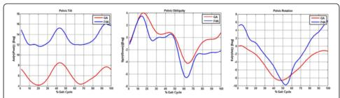
**Figure 4 F4A versus GA: patterns comparison.** Pelvic angles about the three axes, as provided by F4A as the mean of all the detected cycles (blue lines), and those provided by GA in the second trial (red lines), expressed in the laboratory reference frame; patterns from a single representative subject at self-selected speed are shown.
