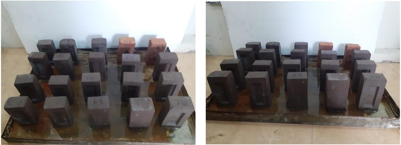
**Figure 15.** Efflorescence of the brick samples.
