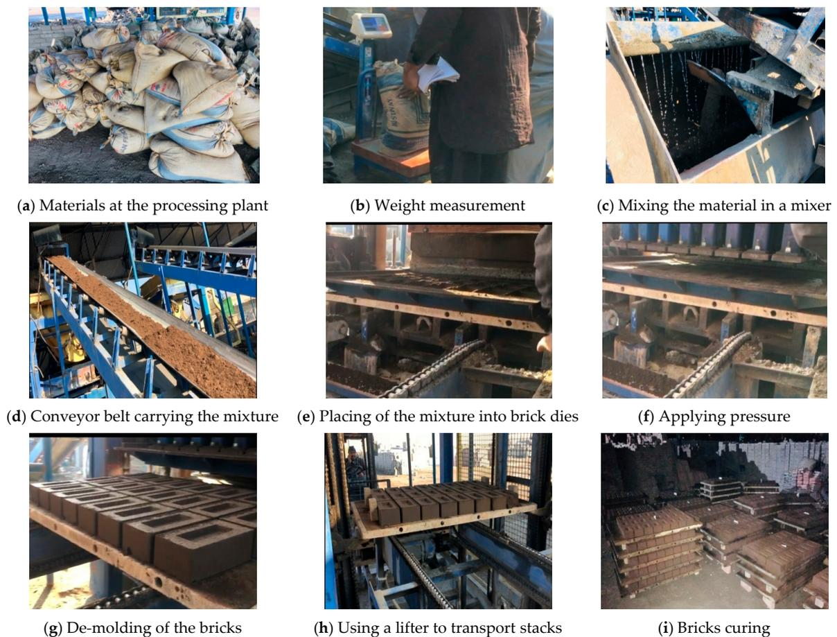
**Figure 2.** The casting process of coal-ash compressed bricks.
