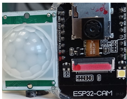
(a) Integrating the ESP-32 AI CAM module with HC-SR501 PIR sensor into a DVN
