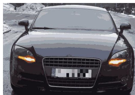
(c) Output image from the K_Means algorithm for K (colors) = 12: Size: 32 approx.
