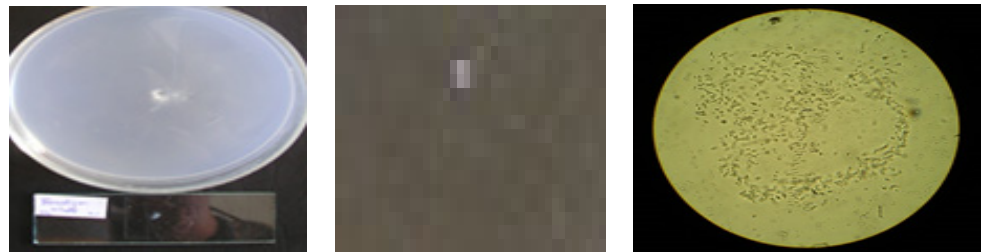
Figure 11. Macroscopic and microscopic images of the APDMS-CL sample on the surface of which the fungus Fusidium viride developed.
