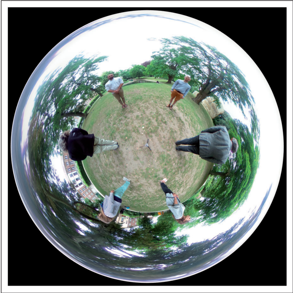
Figure 21. A Postel map based on Riemann normal coordinates centred at the nadir. The whole circular circumference represents the zenith, a single point. This map is neither conformal nor area true. It is quite nice near the origin (the nadir) though, essentially up to the horizon. Distances from the nadir and angles at the nadir are perfectly represented. Notice that the tripod on which the camera was mounted is visible at the centre. The camera cannot see itself. It takes two 190^\circ back-to-back fish-eye photographs and stitches these together in the camera. The output is an equirectangular representation of the full optic array.
