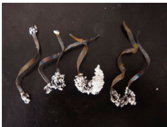
Figure 4. Appearance of stainless-steel strips after microwave discharge [96]. Reprinted from (AIChE Journal, 2012, 58, 3852–3857) with permission from John Wiley and Sons.
