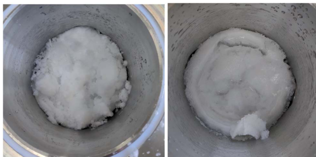
Fig. 10 (A) photos of hydrate formation (degree of under cooling = 4 °C), (B) photos of hydrate formation (degree of under cooling = 2 °C).
