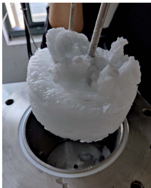
Fig. 6 Photos of hydrate formation (ZIF-8 content = 0.03 \text{ mg mL}^{-1} ).
