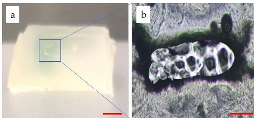
**Figure 10.** Morphology of the channels: (a) the section view of the hydrogel matrix (Scale bar: 4 mm); (b) the section view of a thin sheet of hydrogel matrix containing the channel (Scale bar: 400  $\mu\text{m}$ ).
