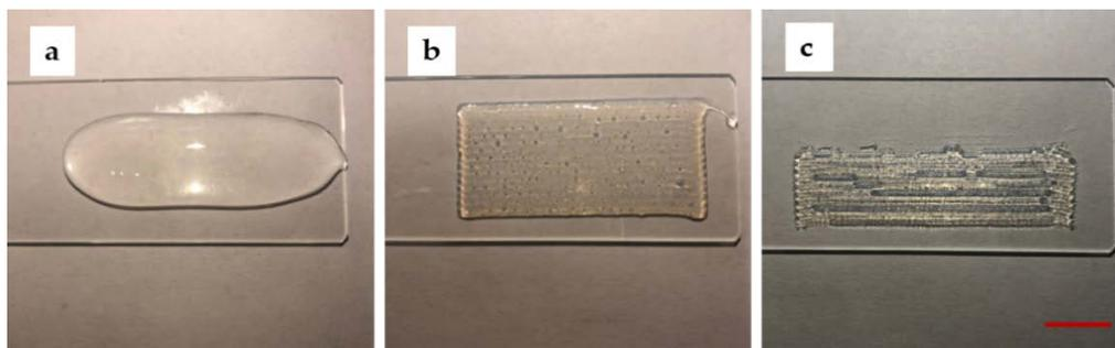
**Figure 2.** The printed results for concentration of sodium alginate are 6%, 8%, and 10% (w/v) from left to right (Scale bar: 1 cm). (a) the printed result for 6% (w/v) sodium alginate; (b) the printed result for 8% (w/v) sodium alginate; (c) the printed result for 10% (w/v) sodium alginate (Scale bar: 1 cm).
