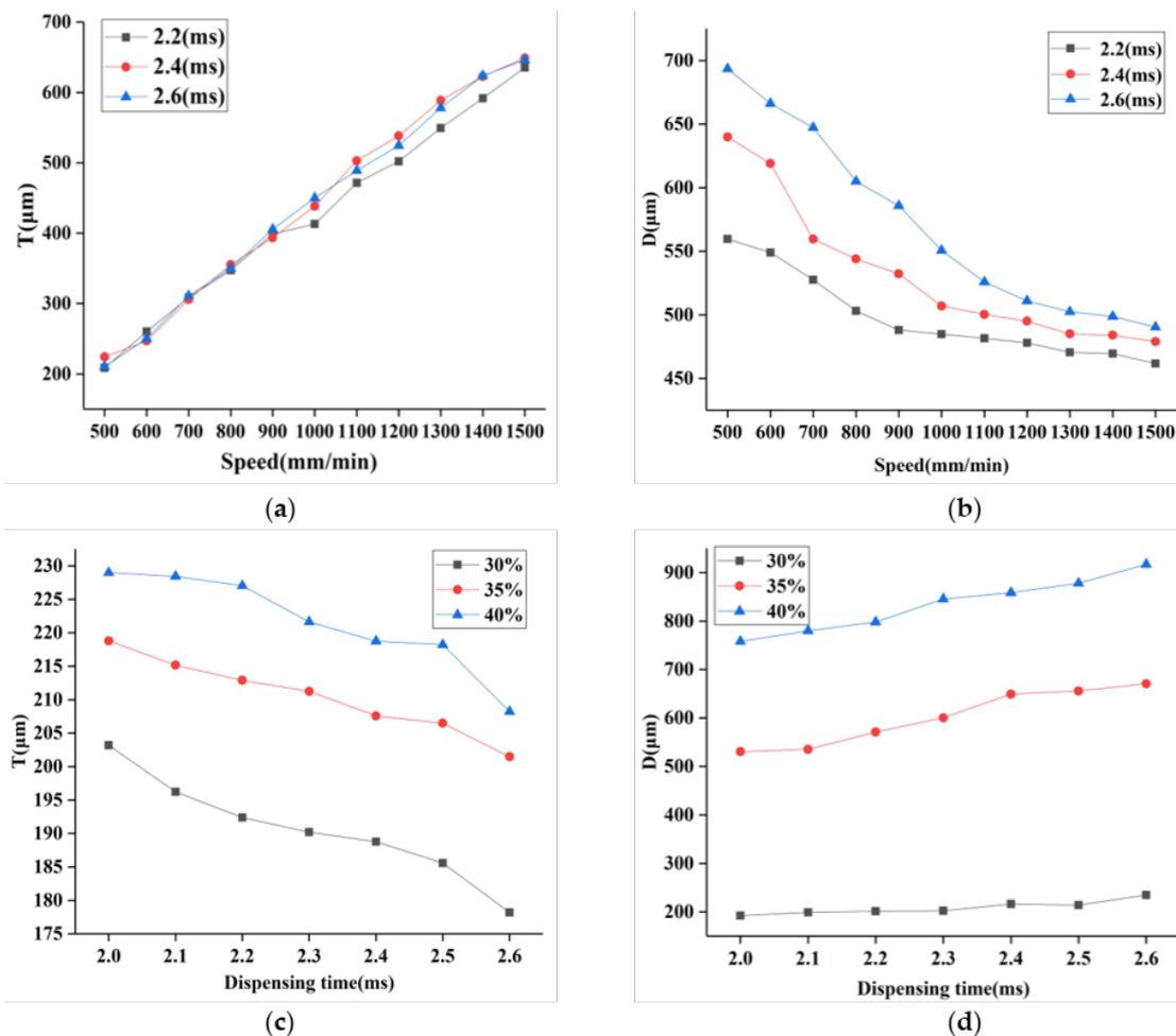
**Figure 5.** Characterization of the printed droplets and lines. (a) Mean spaces of the printed droplets corresponding to the speed at different dispensing time; (b) mean diameters of the printed droplets corresponding to the speed at different dispensing time; (c) mean spaces of the printed droplets corresponding to the dispensing time under different voltage; (d) mean diameters of the printed droplets corresponding to the dispensing time under different voltage.
