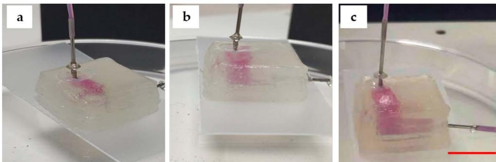
**Figure 9.** Perfusion: (a) the channel is partially perfused; (b) the two connected channels after the perfusion; (c) all channels with 3D structure were perfused with pink deionized water (Scale bar: 1 cm).
