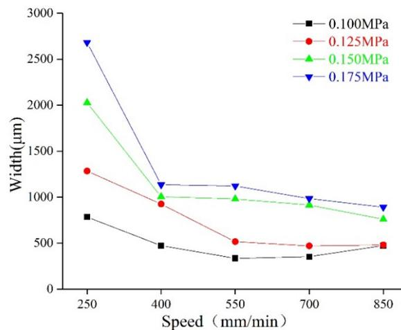
**Figure 3.** The molding relationship: dependence of the combination of extrusion pressure and speed on filament width.
