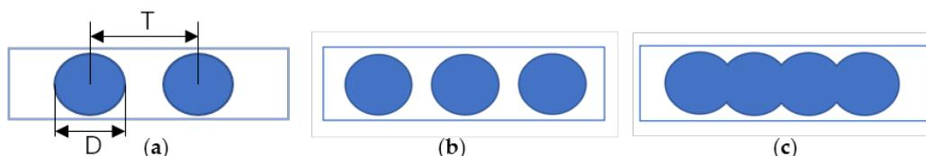
**Figure 4.** Schematic for connecting droplets into a line: (a) the printed droplets of diameter D and space between droplets T; (b) when  $T > D$ , there are gaps between the droplets; (c) when  $T \leq D$ , droplets overlap to form a line.
