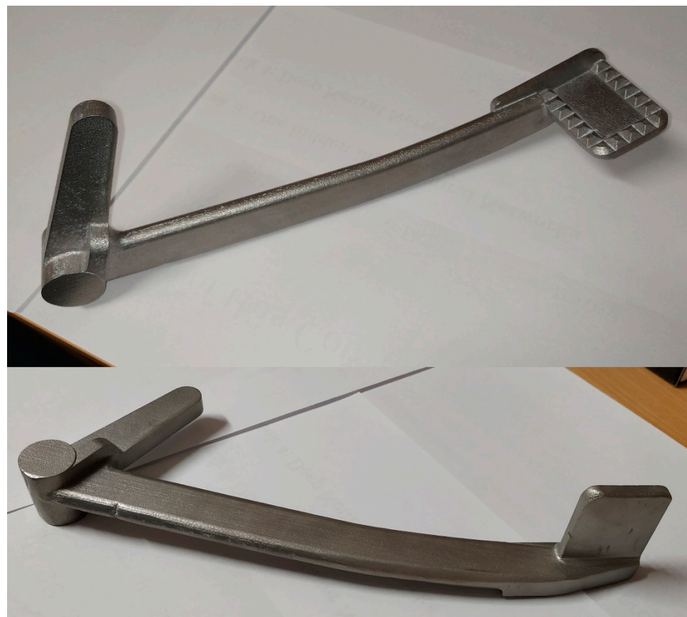
Figure 17. Surface finishing with grinding, sandblasting, and tumbling.
