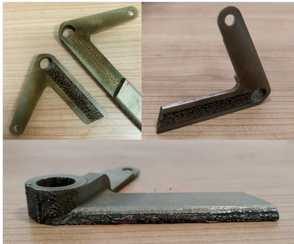
Figure 25. The cut optimized pedal for view into the internal lattice structures.
