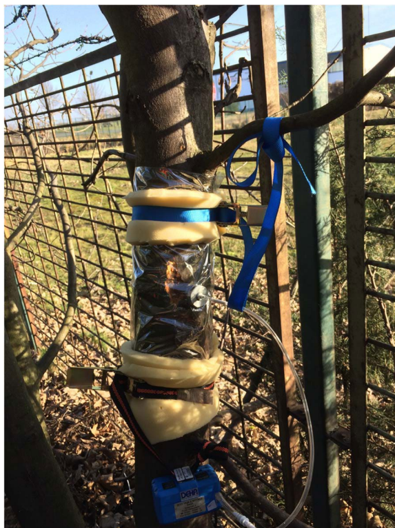
Figure 1. Sampling procedure on a tree trunk. The analysed part is wrapped in Nalophan foil, closed with staples and tension belts.
