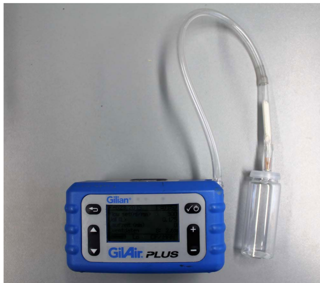
Figure 2. Sampling procedure for beetles, pupae and frass. The samples are stored in the headspace vial while sampling with the pump.
