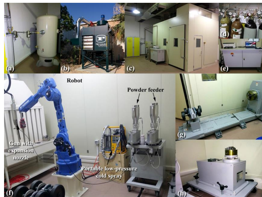
Figure 1. Fully automated cold spray system housed in Nanotechnology Laboratory, KISR used for coating of stainless-steel (SUS 304) sheets with metallic glassy \text{Cu}_{50}(\text{Ti}_{50-x}\text{Ni}_x) alloy powders. The cold spray components are (a) pressurized air reservoir, (b) filtration system, (c) completely sealed cold spray room, (d) argon/nitrogen/compressed air gas cylinders, and (e) control unit, (f) main components including powder feeders, a robot, low-pressure cold spray system for outdoor coating, (g) horizontal turntable, and (h) vertical turntable (for coating the outer and inner parts of the objects).
