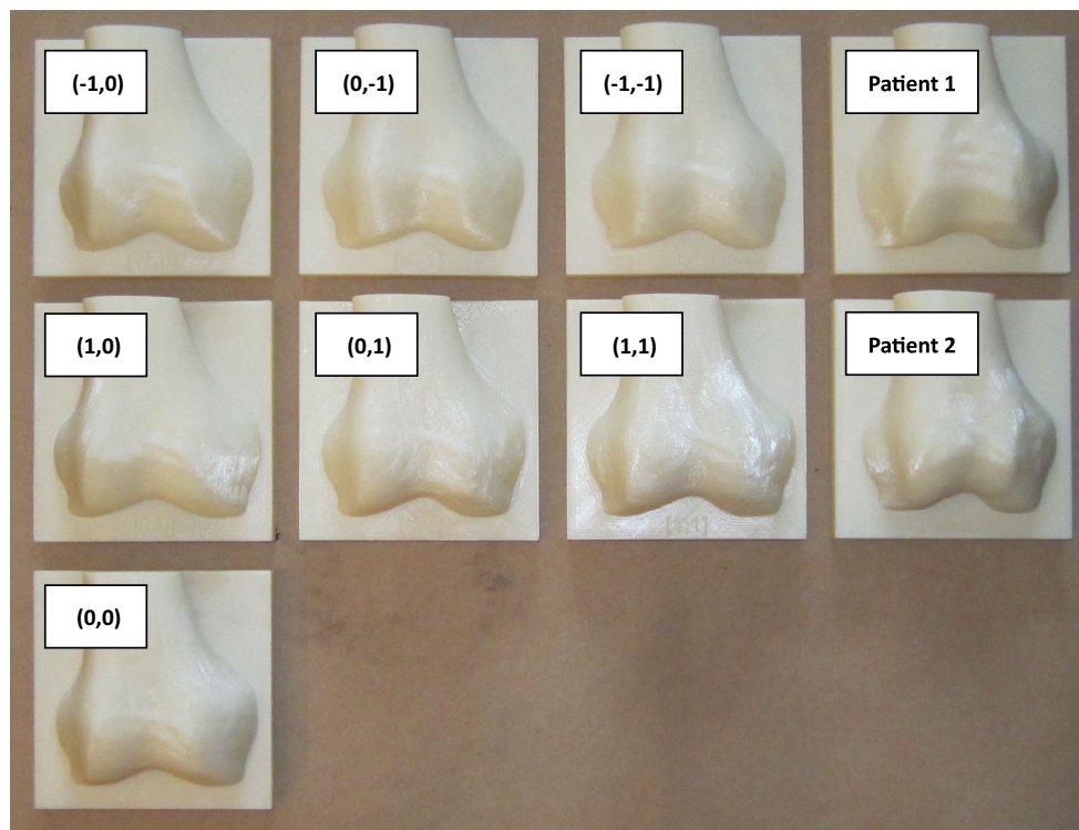
Fig. 13 3D printed distal femora that were used in the experiments
