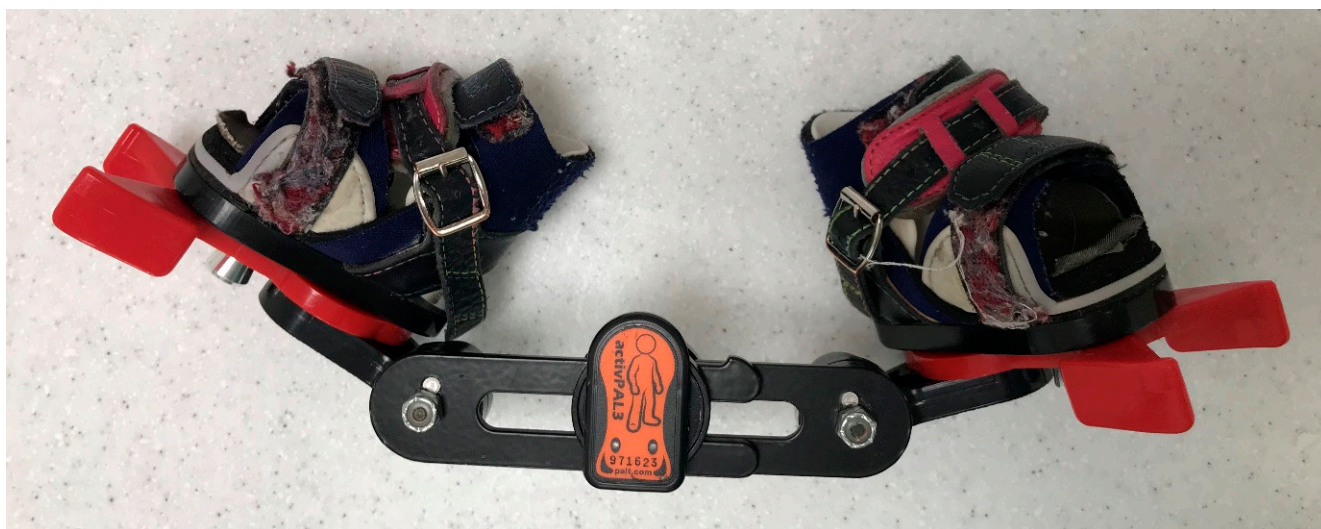
Figure 1. Data collection setup with activPAL PAL3 attached to a FAB.
