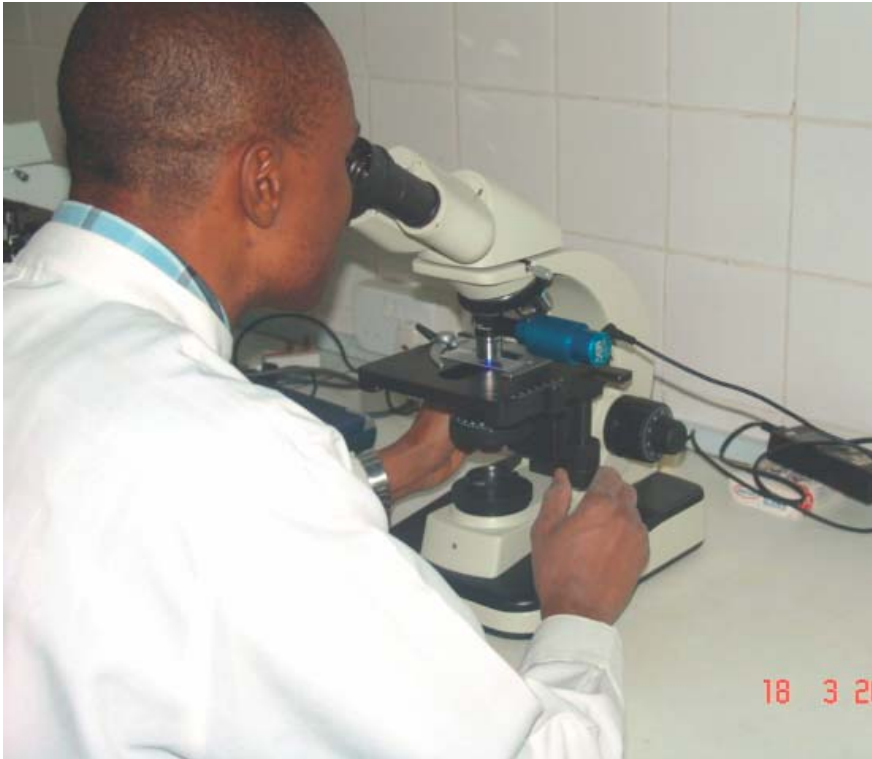
Figure 1. Low-Cost LED-Based Fluorescence Microscopy Being Evaluated at a TDR/WHO Trial Site in Abuja, Nigeria
