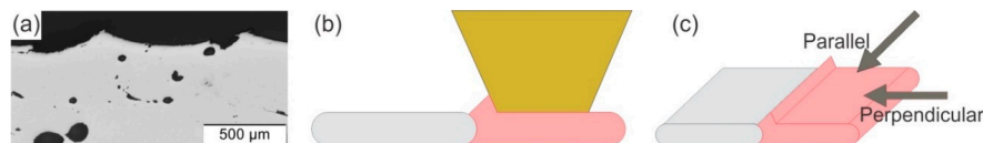
Figure 11. (a) Effect of excessive overextrusion on the top extruded layers; (b) schematics of the origin of the overextrusion defects by the extrusion of a new road of hot material (in red) over a previously deposited road of cold material (in gray); (c) schematics of the material deposition on top of a road with overextrusion if the roads of the new layer are parallel or perpendicular to it.
