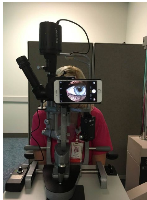
Figure 1. Demonstrating the method of photographing the anterior segment of the eye using iPhone 6.
