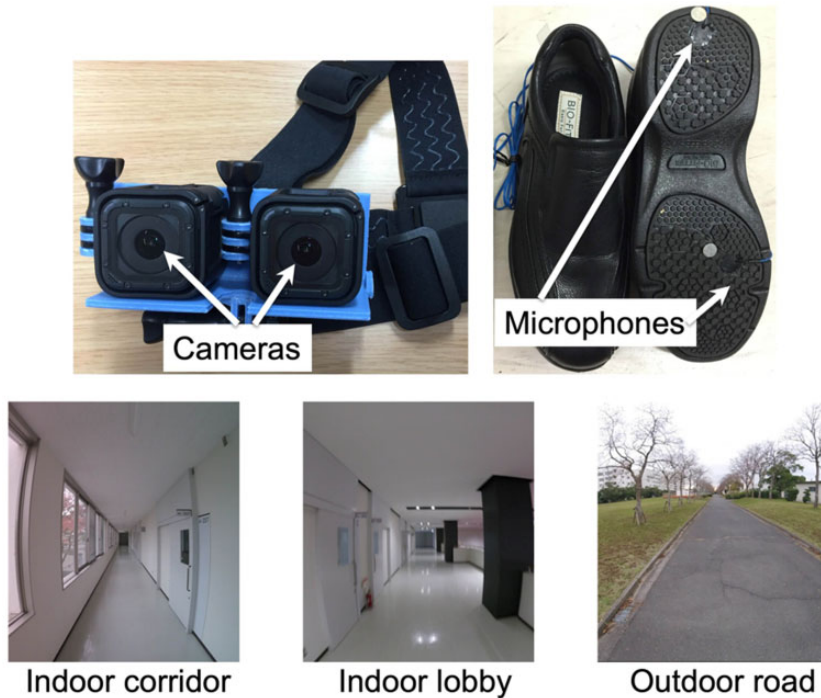
Figure 1. Stereo camera device for capturing stereo motion images (top-left). A pair of shoes with microphones for capturing timings of footsteps (top-right). Three locations where the walking scenes were captured (bottom).
