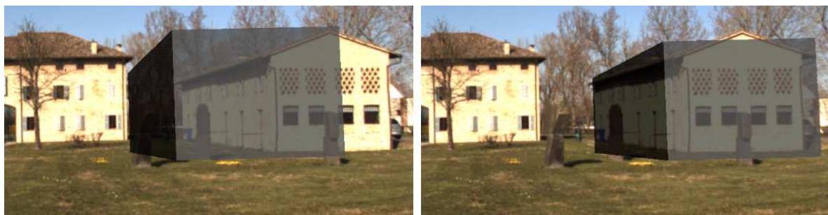
Figure 17. Building visualization in augmented reality: result from coarse registration (left) and after manual correction (right).
