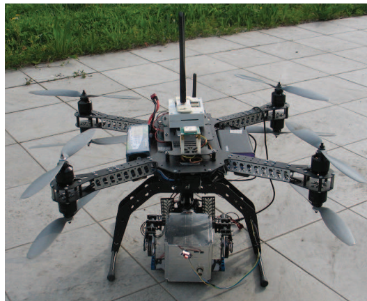
Figure 3. UAV equipped with the CdZnTe gamma-ray detector (mounted at the bottom).
