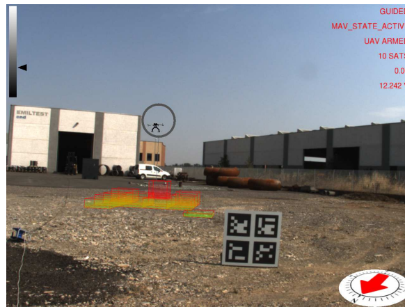
Figure 18. Simulated environment developed for the usability tests. The UAV is a 3D model simulated using the ArduCopter SITL simulator.
