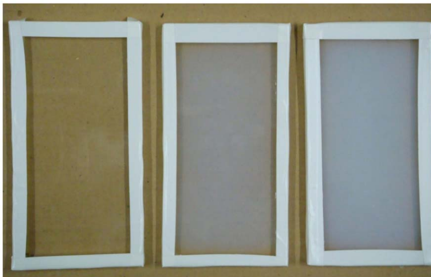
Figure 2. Thin polymer gel cassettes after irradiation. From left to right: 0 Gy (before irradiation), 5 Gy, and 10 Gy.
