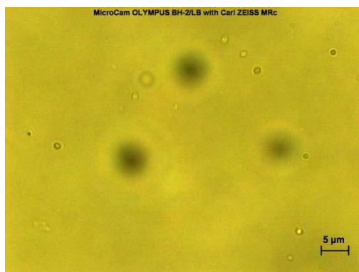
Figure 2. Microfluidic-prepared empty niosomes comprised of Span ® 60, cholesterol, and Cremophor ® ELP.
