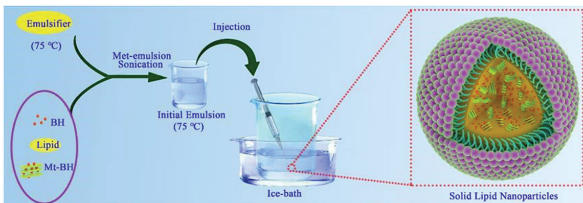
Figure 1. The schematic illustration for the formation of Mt-BH-SLNs. Initial emulsion was obtained by subjecting organic phase containing the emulsifier and the internal aqueous phase containing Mt-BH with met-emulsion sonication. Solid lipid nanoparticles were prepared by injecting the initial emulsion into external aqueous phase with rapid stirring in an ice-water bath.
