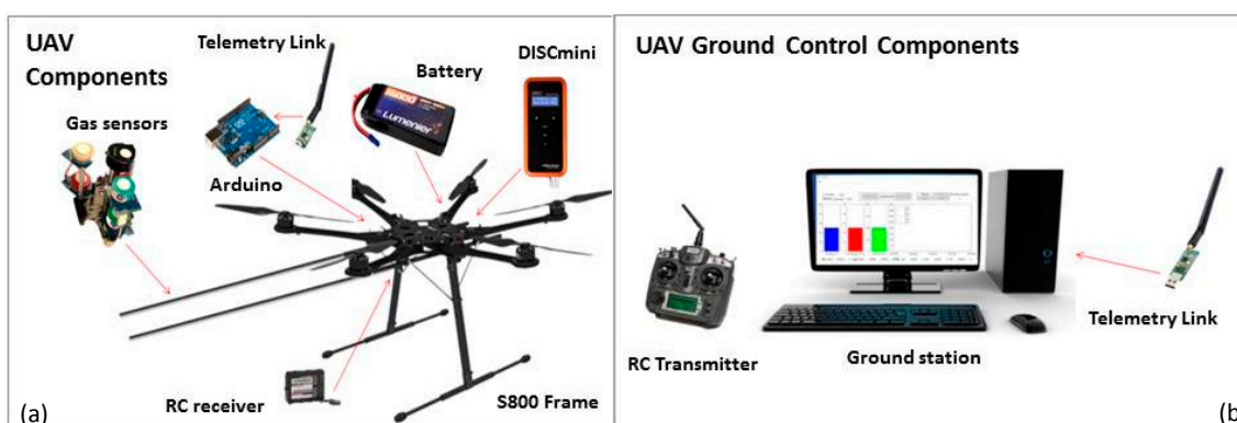
Figure 1. (a) Unmanned aerial vehicle (UAV) system components including gas sensors, DISCmini, Arduino MEGA 2560, battery and RC receiver; (b) UAV Ground Control Components for both manual (using RC transmitter) and autonomous (using PC) operations.
