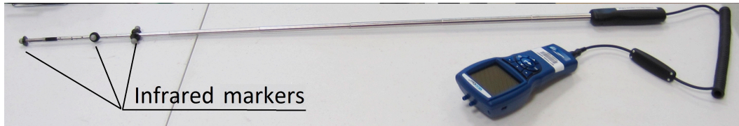
Figure 3. The Portable anemometer TSI, model 9565-P [19] with infrared targets to track and record the anemometer probe position during Test 1 with the VICON system.
