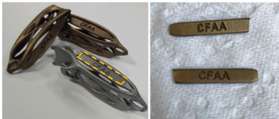
Figure 1. AlTiSiN coated specimens—Set 1.
