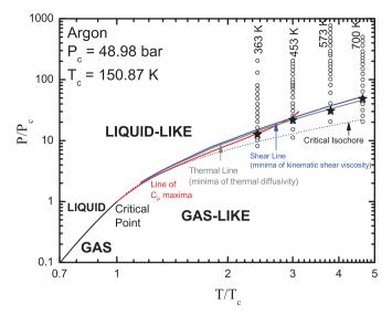
**Figure 4** | Reduced phase diagram (P/Pc -T/Tc) for Argon. Open dots: P-T points used in MD simulations. Stars: onset of PSD at the four isotherms, based on linear extrapolation of the PSD data points to low densities (see figure 2). Lines (obtained from NIST<sup>23</sup>): loci of the extrema of  $c_P$  (red),  $D_T$  (grey) and v (blue). Dotted line: critical isochore.
