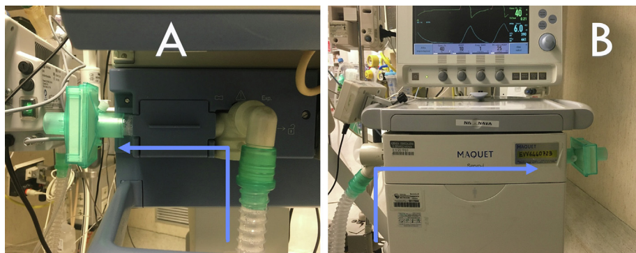
Fig 1. High efficiency particulate filters placed after ventilator expiratory valve (A: Dräger Evita XL, B: Getinge Maquet Servo I).
