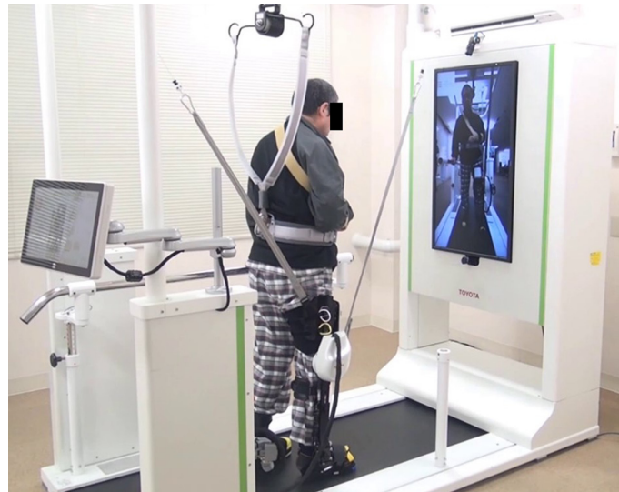
Fig. 1. The Gait Exercise Assist Robot (GEAR).
