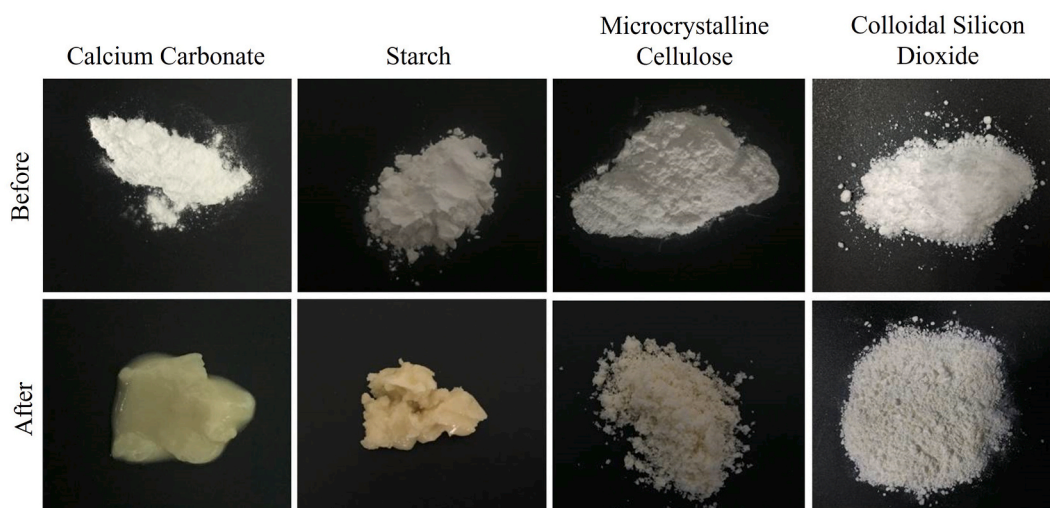
Fig. 1. Appearance of different adsorbents before (upper) and after (lower) mixed with Patchouli Oil.
