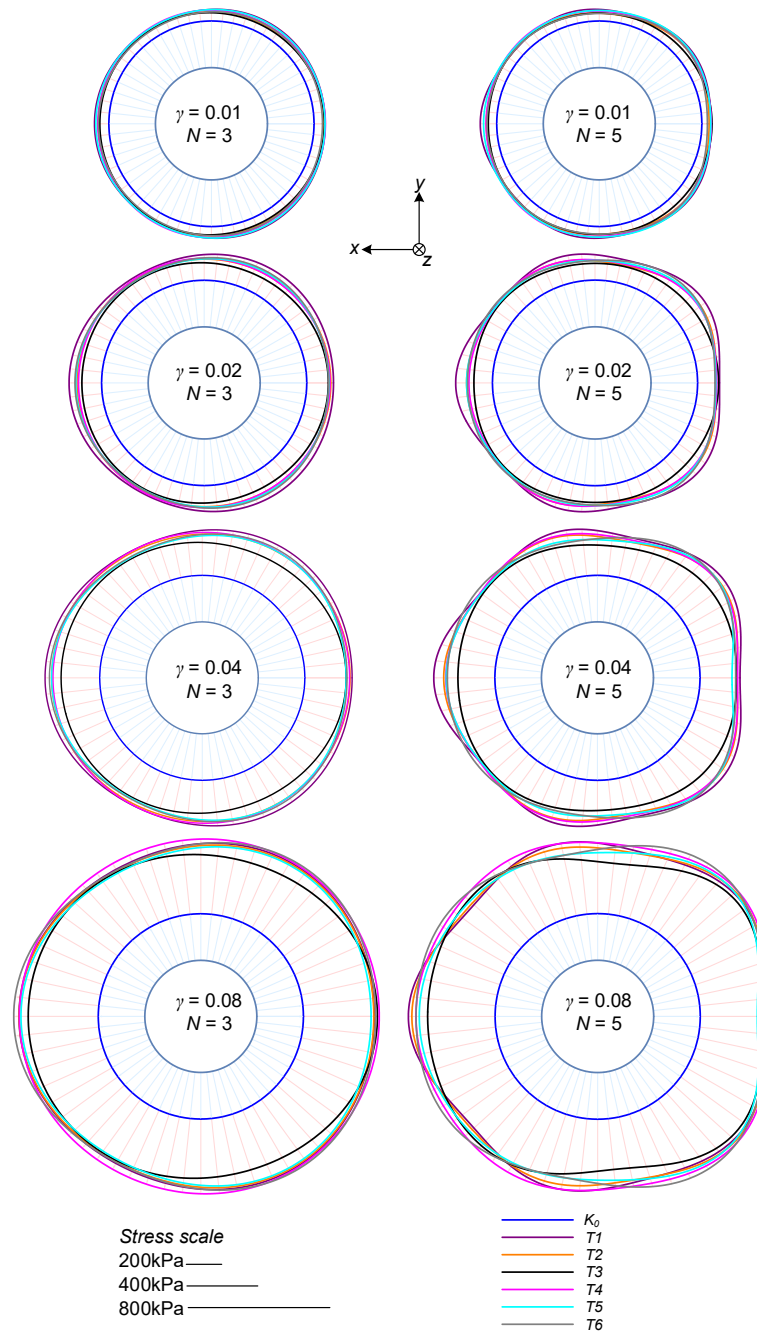
Figure 9. Contact stress distributions at different stages of the shear tests.
