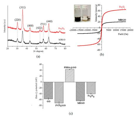
**Figure 4.** (a) XRD pattern and (b) VSM curves for  $Fe_3O_4$  and MRGO; and (c) zeta potential for various as-prepared graphene and  $Fe_3O_4$ .
