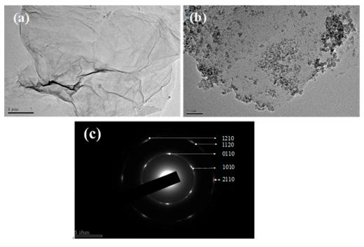
**Figure 2.** TEM image of (**a**) graphene oxide (GO) (scale bar: 1 mm); (**b**) MRGO (scale bar: 50 nm); (**c**) selected area electron diffraction (SAED) pattern of GO.
