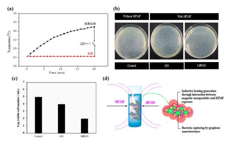
**Figure 7.** (a) Inductive heating temperature of GO and MRGO by high frequency magnetic field (HFMF); (b) bacteria activity with and without HFMF exposure; (c) survival *S. aureus* numbers of GO and MRGO by HFMF; (d) schematic diagrams of bacteria capturing activity and HFMF exposure.
