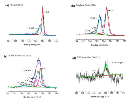
**Figure 3.** XPS spectra (C-1s) of (**a**) graphite, (**b**) graphene oxide (GO), (**c**) GO-poly (diallyldimethylammonium chloride) (PDDA) (RGO), and (**d**) XPS (N-1s) of GO-PDDA (RGO).
