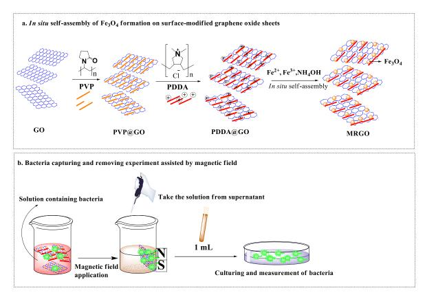
**Figure 1.** Schematic diagram of (**a**) magnetically reduced graphene oxide (MRGO) preparation and (**b**) bacteria capturing and separation assisted by magnetic field.
