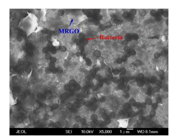
Figure 6. SEM image of MRGO sheets capturing bacteria (S. aureus) (scale bar: 1 µm).
