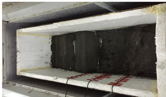
Figure 3. Pile-up process of tailings dam model.
