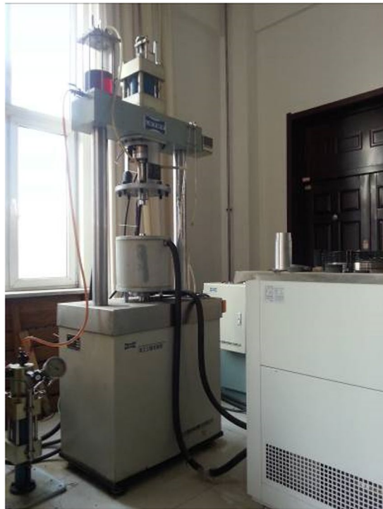
Figure 2. Permafrost triaxial testing machine.
