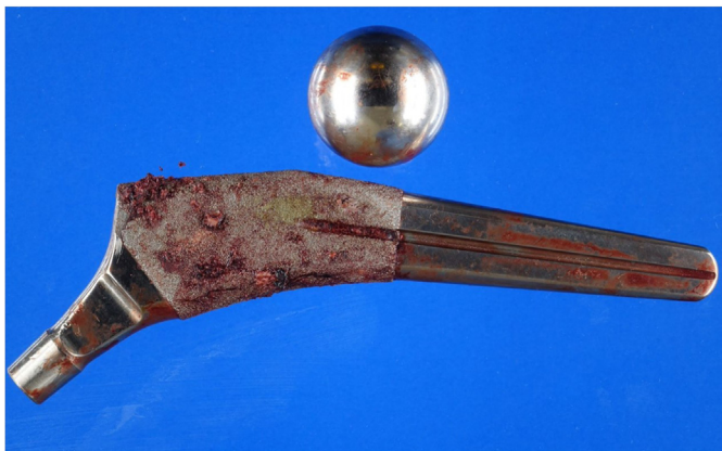
Figure 3. A cementless stem removed during revision to a long fully porous femoral implant. Note the exposed on-growth surface and fragments of attached bone, for bone-to-implant and bone-to-bone healing.
