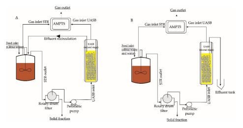
**Figure 1.** Schematic figure of the semi-continuous two-stage system with liquid recirculation (**A**) and without recirculation (**B**) (modified from Aslanzadeh et al. [20]). AMPTS = Automatic Methane Potential Testing System; STR = Stirred tank Reactor; UASB = up-flow anaerobic sludge blanket.
