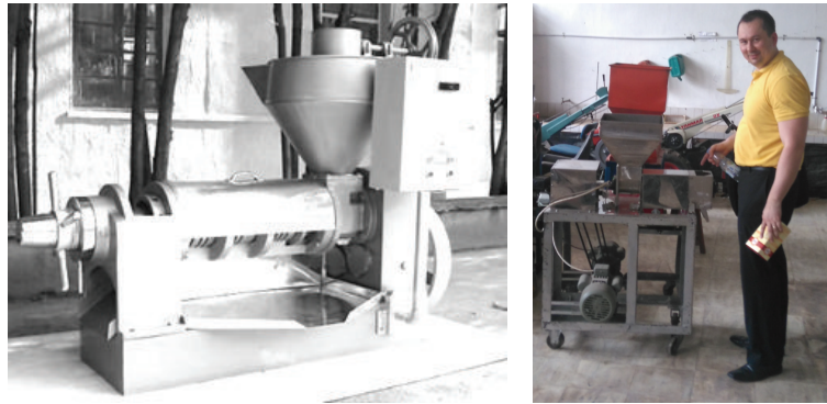
FIGURE 2: Typical machines mechanically extracting oil from Jatropha curcas L. seeds.
