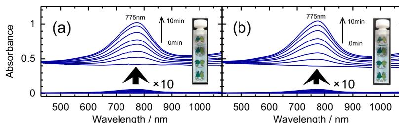
**Figure 3.** Typical absorption spectral changes of (a) as-prepared  $\text{WO}_3$  and (b)  $\text{TM}\beta\text{CDx}/\text{WO}_3$  binary aqueous solution under UV light irradiation. Concentration conditions:  $[\text{WO}_3] = 1.0 \times 10^{-2}$  M,  $[\text{TM}\beta\text{CDx}] = 1.0 \times 10^{-2}$  M,  $[\text{Na}_2\text{SO}_4] = 3.3 \times 10^{-2}$  M, pH 1.5. The insets show the photograph of the sample solutions after the irradiation for 30 min.
