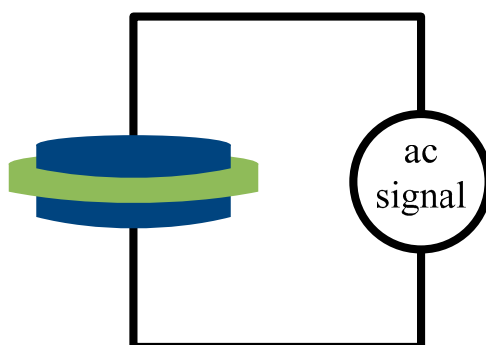
Figure 8. Schematic diagram for electrochemical stability measurement.
