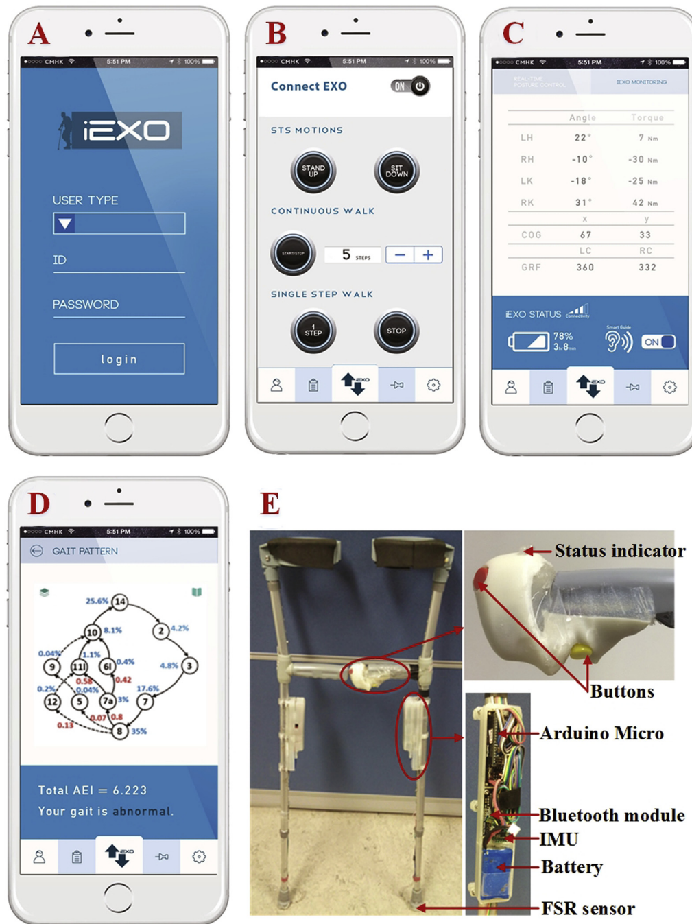
Figure 2 Human–machine interface of CUHK-EXO. (A) Login In view of smart phone App; (B) Operation view of smart phone App; (C) Motion Monitoring view of smart phone App; (D) Performance Evaluation view of smart phone App; (E) design of the smart crutches. App = application; FSR = force-sensing resistor; IMU = inertial measurement unit.
